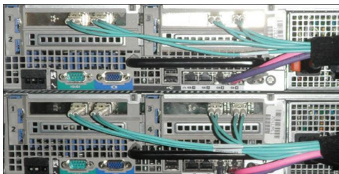
Figure 2. Simplified server connectivity using 10GbE
